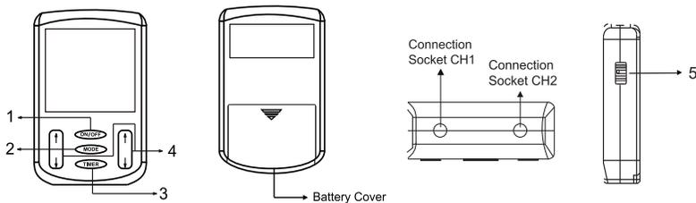
1. ON/OFF Button: Turns the power on and off.
