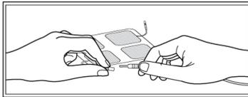
**Note:** Use care when you plug and unplug the wires. Pulling on the lead wire instead of its insulated connector may cause wire breakage.
